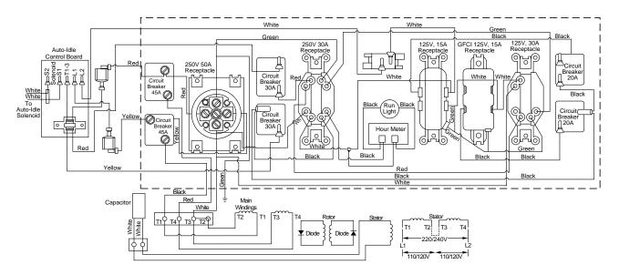
Figure 35 - Wiring Diagram, Model RGH11000AIE
